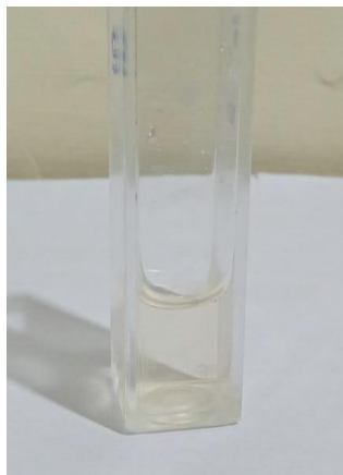
Figure 35. Melamine detection in milk using DRE AgNPs (0 minutes).
