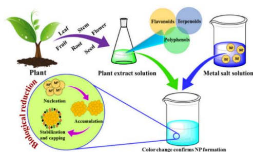
Figure 2. Mechanism of plant extracted mediated green synthesis. 10
